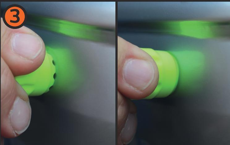
3 Position the SensorCut and cut out the PDC-Sensor
