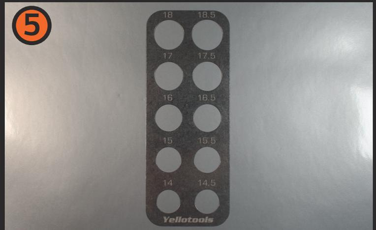
5 Use the template to cut out the desired size
